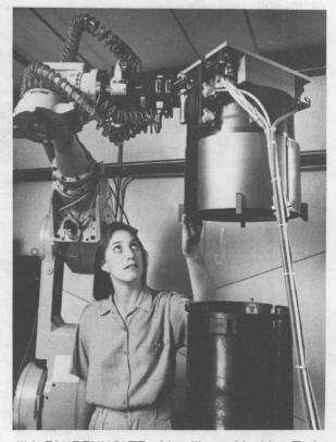
JILL FAHRENHOLTZ of Intelligent Machine Technologies Div. 1416 examines a robotic system under development at Sandia that will help disassemble decommissioned nuclear weapons. Disassembly work is expected to increase as the US reduces its nuclear weapons arsenal. (See "Disassembly Robot Helps Scale Up US Weapons 'Build-Down.'")
